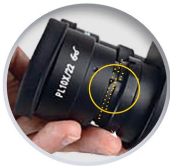
Bayonet locking mechanism on eyepiece ensures that the reticle remains orthogonal with the polarizer and analyzer.
