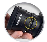
Bayonet locking mechanism on eyepiece ensures that the reticle remains orthogonal with the polarizer and analyzer.
